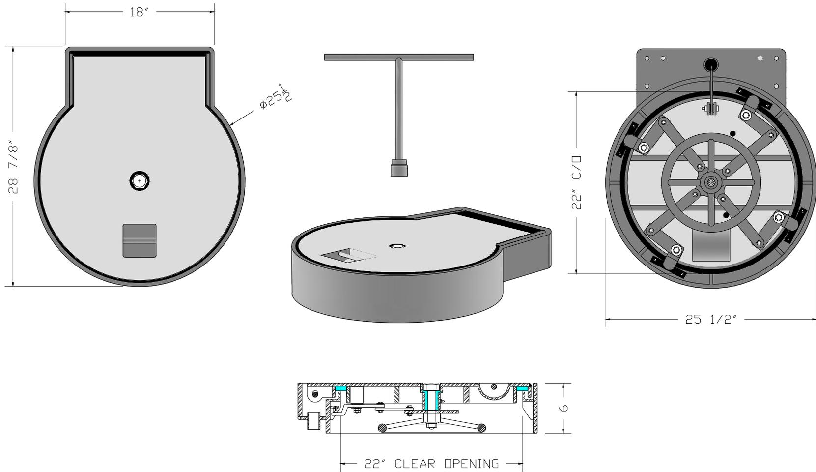
HATCH COVER IS SPRING ASSISTED (NOT SHOWN)
